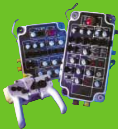
Challenger 2 gunner's & commander's panels and gunner's control handle
